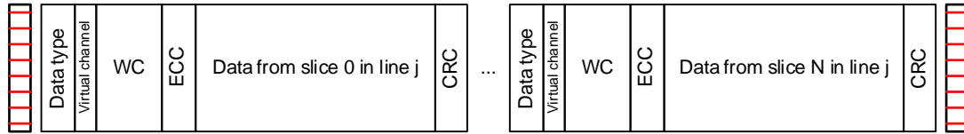
Figure 41 One Line Containing More than One Compressed Pixel Stream Packet
